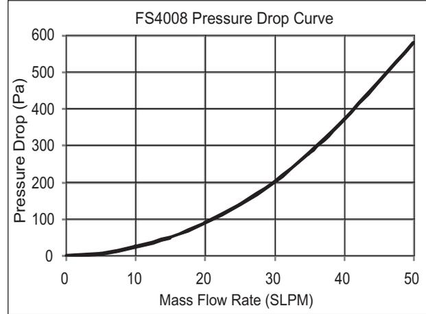
Figure 1.4: FS4008 pressure drop v.s. flow rate.
