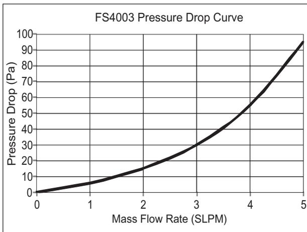
Figure 1.3: FS4003 pressure drop v.s. flow rate.
